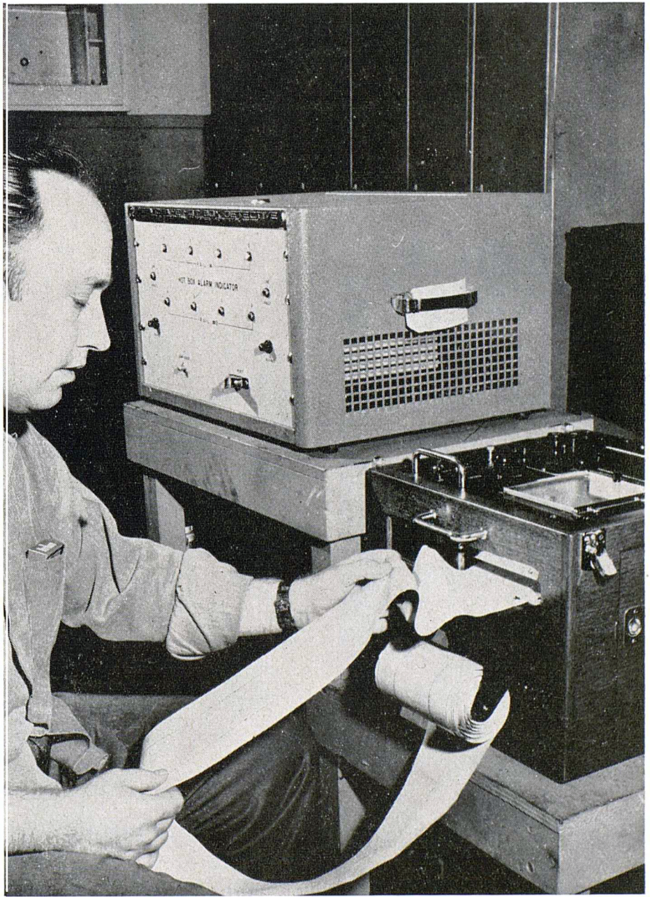
3 Nest block operator is alerted by buzzer and a red indication lamp that train has an overheated journal. He reads the graph to find the location so he can tell the train crew.
